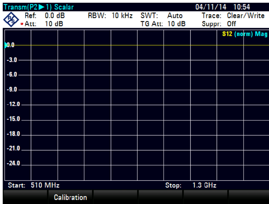
Fig. 2-15: Measurement of a through connection after calibration.
