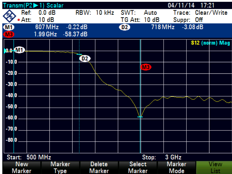
Fig. 2-17: Measurement of the 3 dB cutoff frequency and the maximum stopband attenuation on a lowpass filter.
