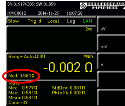
Fig. 2-11: Display of the offset value after calibration.
