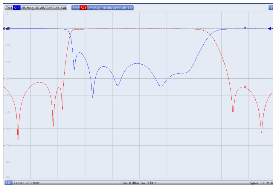
Fig. 5-8: Reflection and transmission in one diagram.
