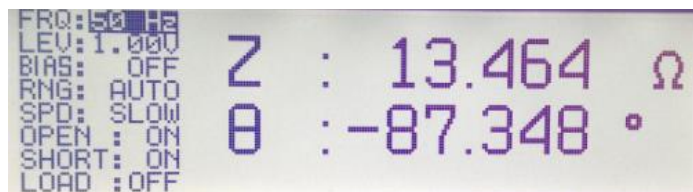
Fig. 2-3: Display of impedance and phase angle for a capacitor.
