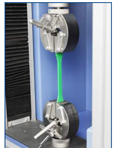
MecS622-BV: Tooth pitch 1.2 mm, hardened steel
