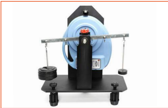
Checks gauge torque cells
