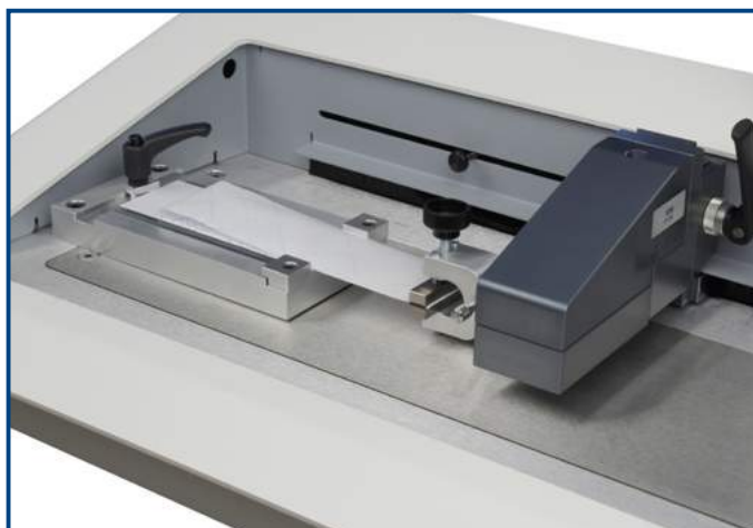
180° peel of self-adhesive labels (with part no. 432-636) ▲
