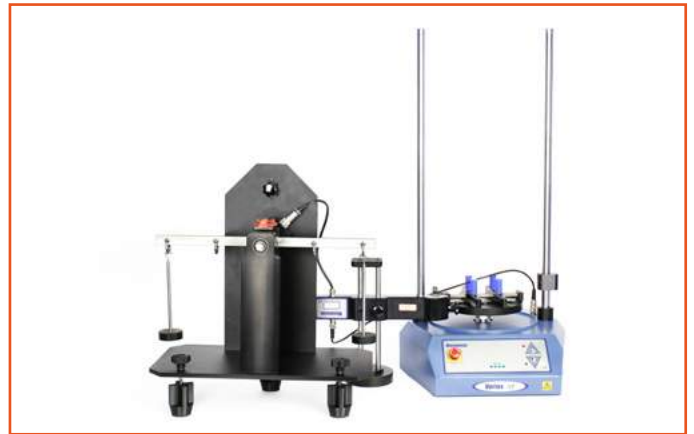
Checks Vortex torque sensors
