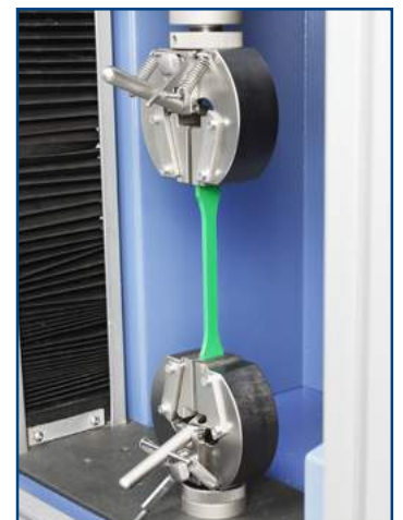
MecS622-BV: Tooth pitch 1.2 mm, hardened steel
