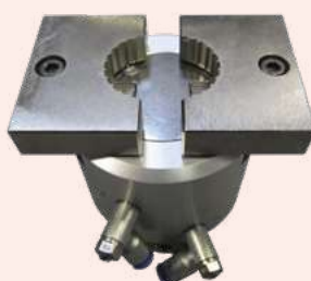
▼ Split mandrel with pneumatic chuck to tighten serrated jaws
