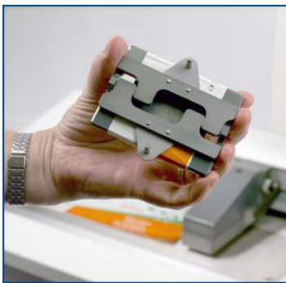
▲ 432-638: 200 g foam faced: ASTM D1894, ISO 8295
