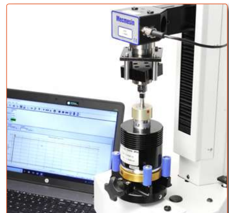
Torque value check on Helixa
