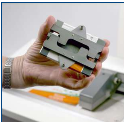
▲ 432-638: 200 g foam faced: ASTM D1894, ISO 8295
