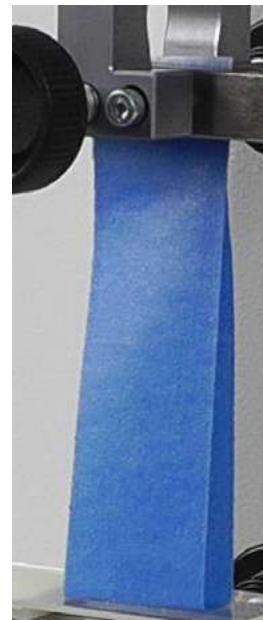
◀ Test Plate (PDV13016-A) shown with 25 mm strip being held in Upper Grip (Mec227-BG50)
