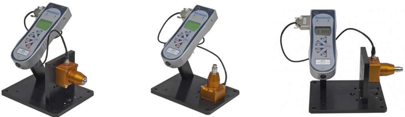
432-401 shown with AFTI mounted and sensor in vertical and horizontal orientation
