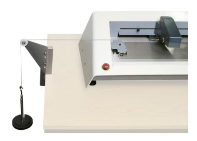
432-635 Pulley jig clamped to bench-top and calibrated weights applied for loadcell accuracy verification
