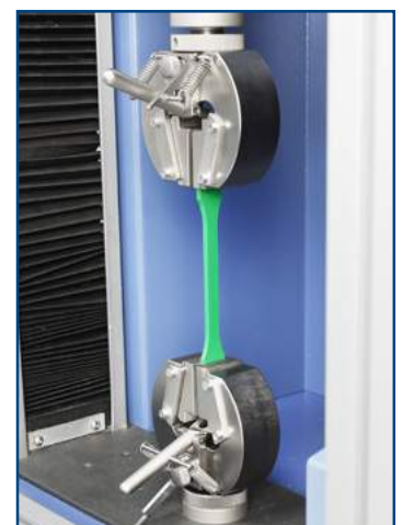
MecS622-BV: Tooth pitch 1.2 mm, hardened steel
