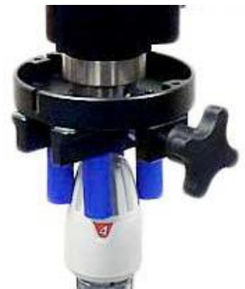
432-321 Upper Fixing Table and 432-447 Pegs gripping a thermostatic radiator valve control
