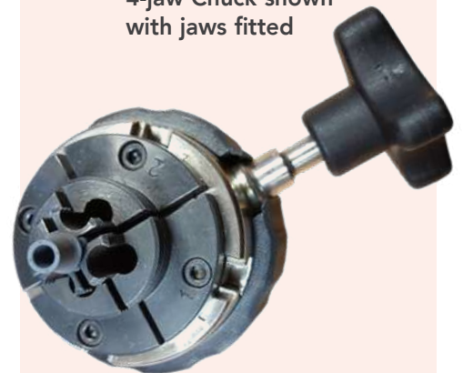
▲ Upper 'key-operated' 4-jaw chuck shown with key fitted and specimen held in mini-jaws
