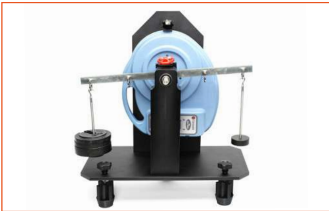
Checks gauge torque cells
