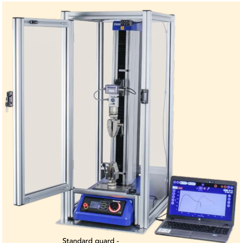
Standard guard - single column test stands ▲
