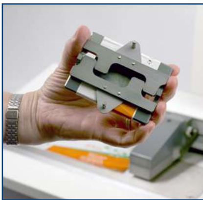
▲ 432-638: 200 g foam faced: ASTM D1894, ISO 8295
