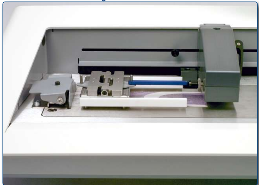
▼ 432-628: 800 g sled shown with ISO 15359 friction test kit
