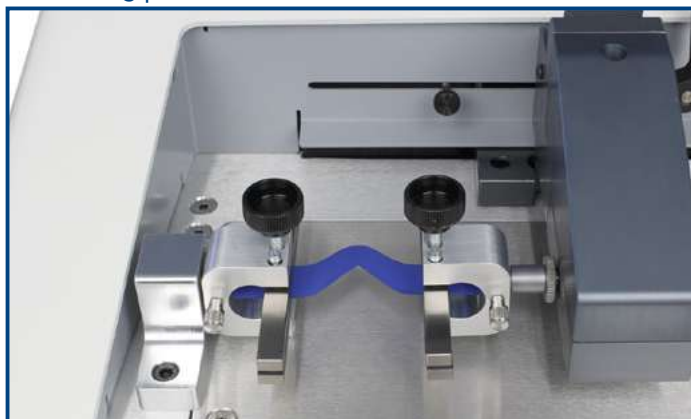
Tear-testing plastic film ▼
