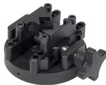
432-600 Precision Lower Fixing Table and 432-602 V-jaws
