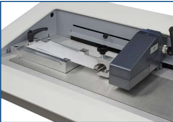
180° peel of self-adhesive labels (with part no. 432-636) ▲
