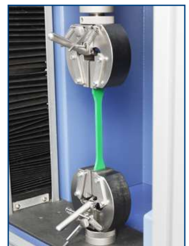
MecS622-BV: Tooth pitch 1.2 mm, hardened steel
