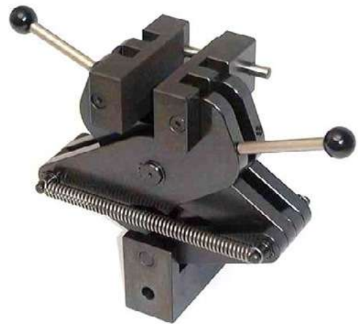
Mec11-50 with Mec11-50-BP pyramid jaws
