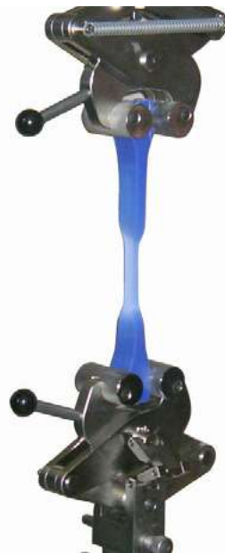
Mec11-20 with Mec11-20-BR jaws shown testing dumbbell specimen
