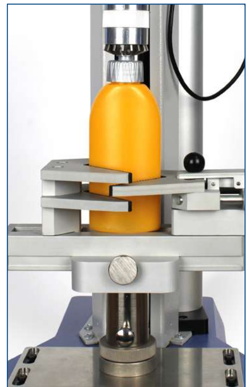
▲ 432-677 Pull-up force to open the spout of a closure
