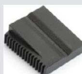
Mec243-BV -V-jaws • For all kinds of round samples • Hardened steel 58 HRC • Tooth pitch 1.2 mm
