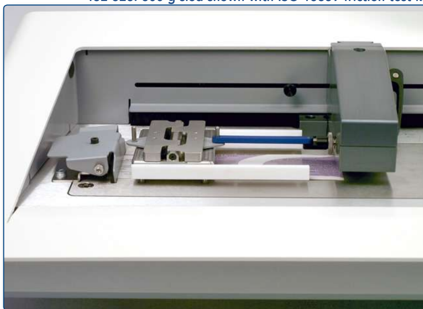
▼ 432-628: 800 g sled shown with ISO 15359 friction test kit
