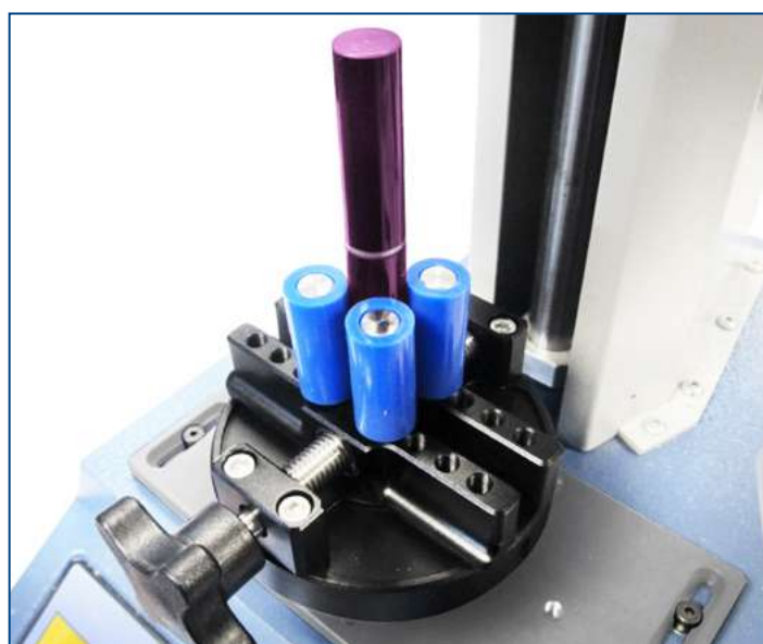
▲ 432-493 Small 4-peg container holder, cosmetics applicator pull-off test
