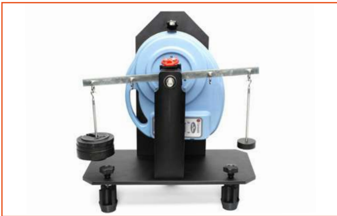
Checks gauge torque cells
