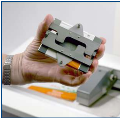
▲ 432-638: 200 g foam faced: ASTM D1894, ISO 8295
