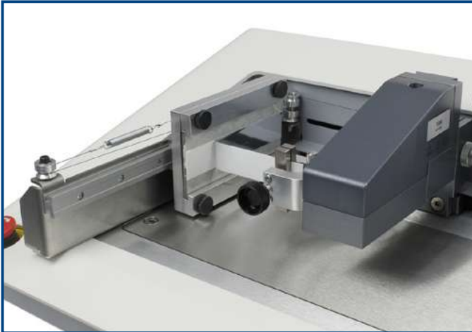
90° peel of laminated card (with part no. 432-620)▲
