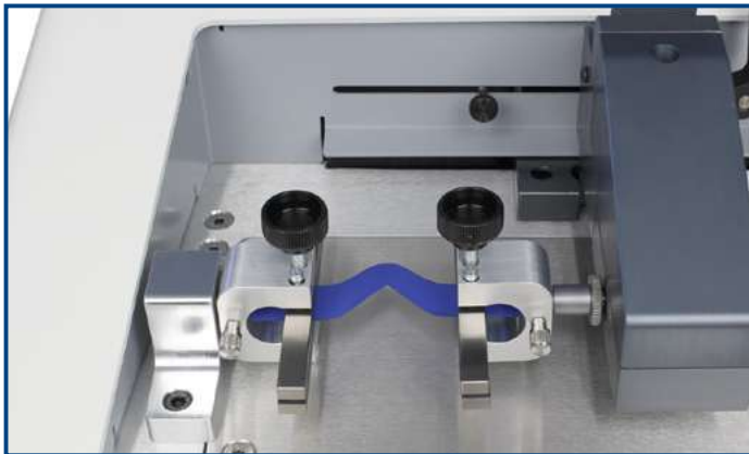
Tear-testing plastic film ▼
