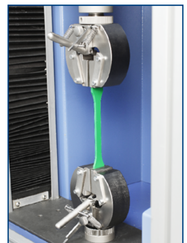
MecS622-BV: Tooth pitch 1.2 mm, hardened steel
