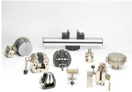
Selection of grips ideal for materials testing
