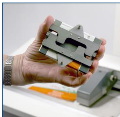
▲ 432-638: 200 g foam faced: ASTM D1894, ISO 8295
