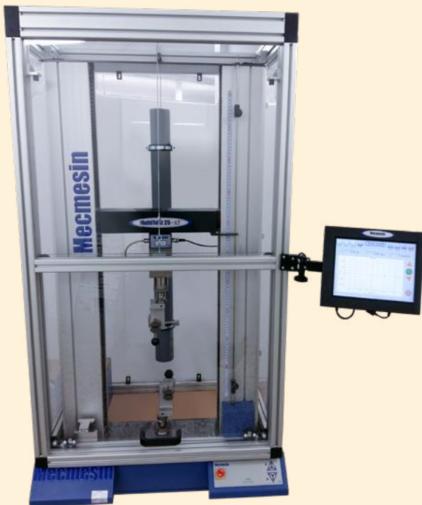
Custom guard with sliding front protective panel and counter-balance for ease of use ▲
