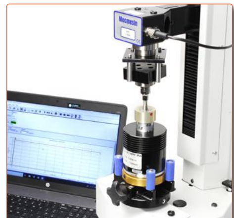
Torque value check on Helixa
