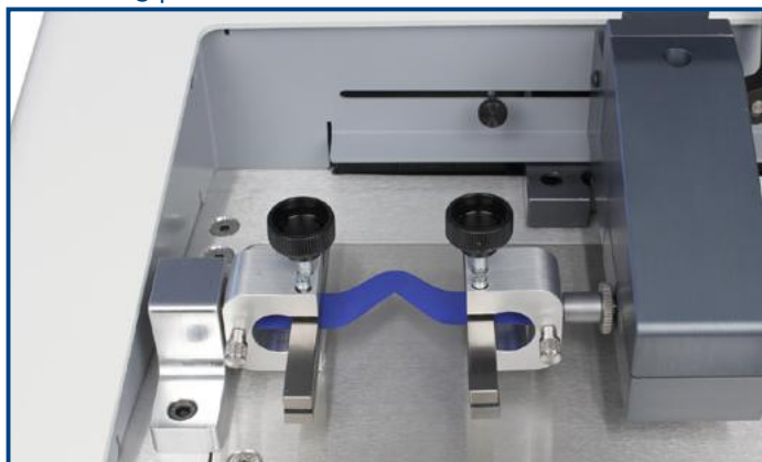
Tear-testing plastic film ▼
