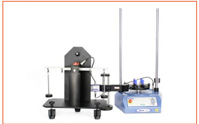
Checks Vortex torque sensors
