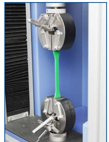
MecS622-BV: Tooth pitch 1.2 mm, hardened steel
