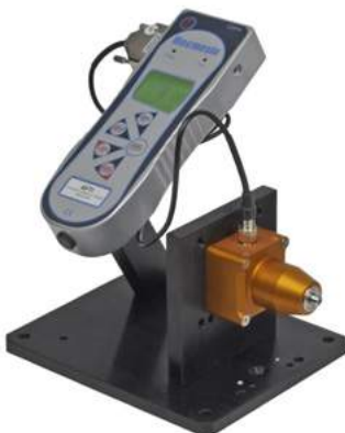
432-401 shown with AFTI mounted and sensor in vertical and horizontal orientation
