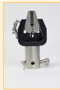
e.g. QC Type K Female sleeve with wedge grip
