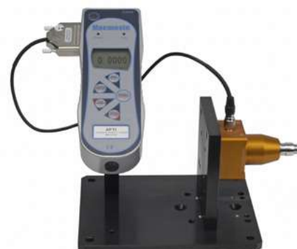
432-401 shown with AFTI mounted and sensor in vertical and horizontal orientation
