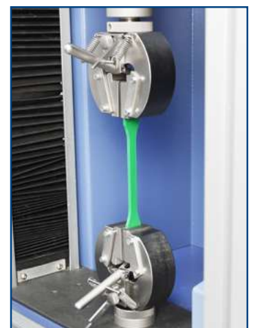
MecS622-BV: Tooth pitch 1.2 mm, hardened steel
