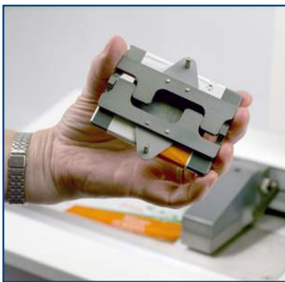
▲ 432-638: 200 g foam faced: ASTM D1894, ISO 8295
