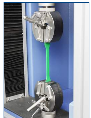
MecS622-BV: Tooth pitch 1.2 mm, hardened steel
