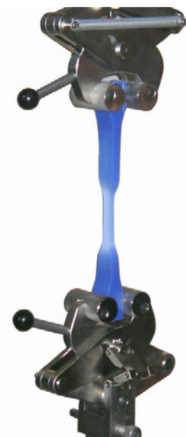
Mec11-20 with Mec11-20-BR jaws shown testing dumbbell specimen
