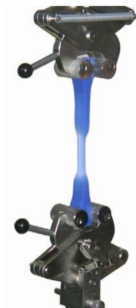
Mec11-20 with Mec11-20-BR jaws shown testing dumbbell specimen
