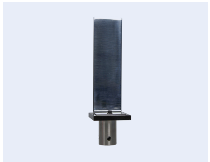
▲ Test Plate (PDV13016-C) for connection to a QC-20 Fixing Post of test stand
