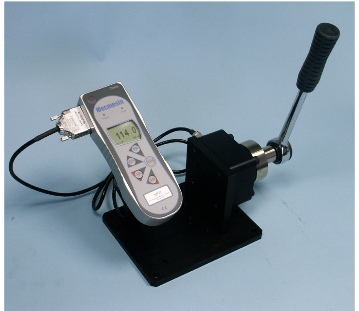
TWC shown testing a mechanical torque wrench
