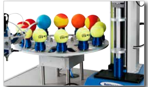
Tennis ball carousel used with a Mecmesin tester
