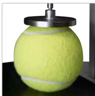
Tennis ball compression test
