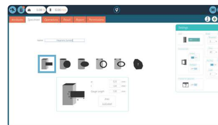
▲ Select the appropriate form of your specimen and the extensometer setting
