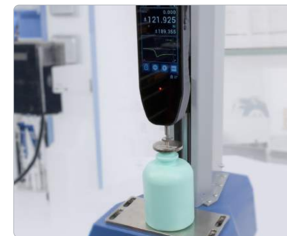
▲ Testing compressive resistance of cosmetic container
