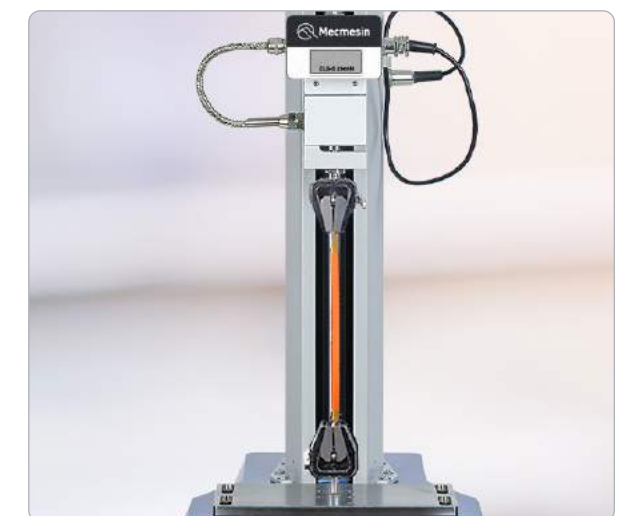
▲ Tensile strength measurement of plastic tubing
