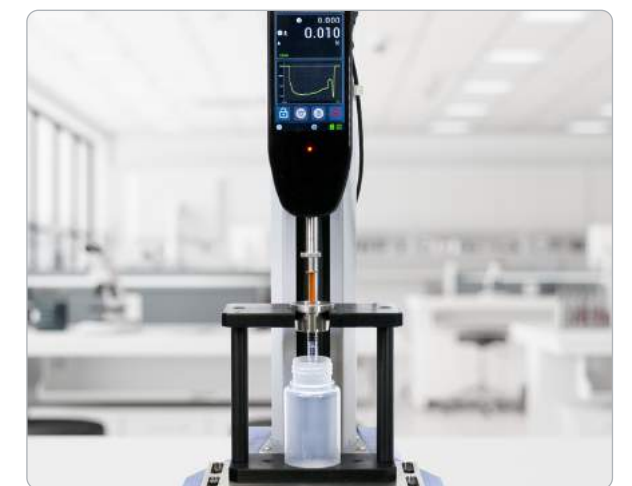
▲ Testing glide force of syringe plunger
