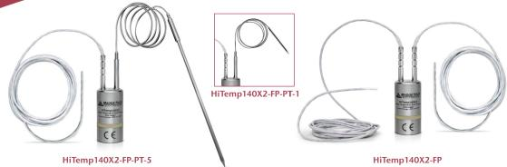
The HiTemp140X2-FP series of dual probe high temperature data loggers are comprised of a stainless steel data logger body and offers four sizes (6 inch, 12 inch, 36 inch and 72 inch) of flexible FP probes or are available with one flexible probe and a stainless steel bendable PT probe combination.
