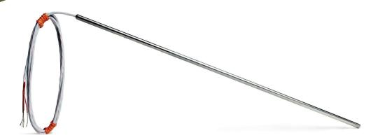
The standard RTD probes are compatible with a variety of MadgeTech data loggers. The series of standard RTD probes are 4-wire, 100 Ohm platinum sensors with a metal strain relief. The metal strain relief is located at the junction of where the lead wire meets the probe and adds another level of protection at this location. The probe series is available in a  $6'' \times 3/16''$  diameter or a  $12'' \times 3/16''$  diameter sheath model, both with a 36'' lead wire.
