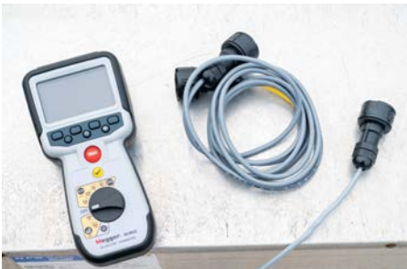
Figure 6-9: A DLRO is a simple but powerful handheld tool capable of taking highly accurate continuity measurements.
