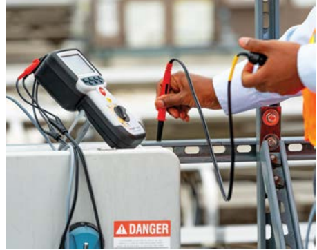
Figure 6-14: DLROs typically have a CAT III safety rating to help protect technicians while they are using the tools.
