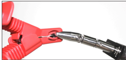
Megger clip being tested with IEC standard test finger to verify touch-proof contact.
