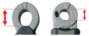
An elliptical shaped head can allow much easier access to ground electrodes in recessed wells.
