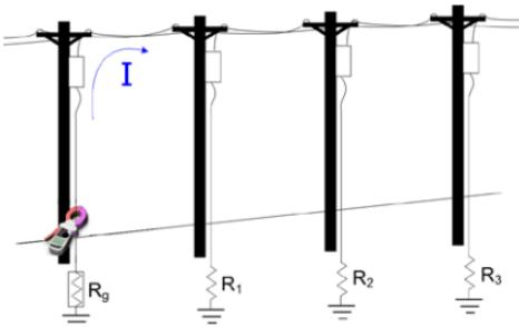
$$R_{eq} = (R_1 \parallel R_2 \parallel R_3 \dots \parallel R_n)$$
