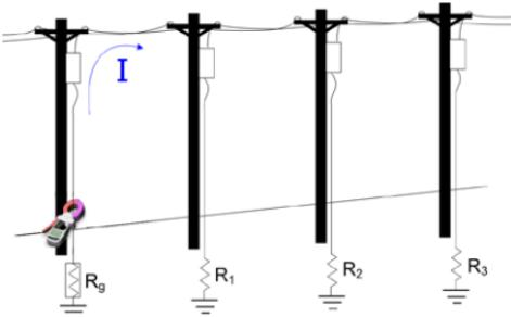
$$R_{eq} = (R_1 \parallel R_2 \parallel R_3 \dots \parallel R_n)$$
