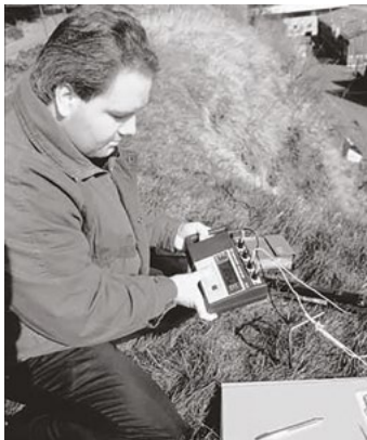
Figure 1: Placing ground testing probes
