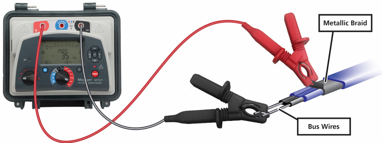
Megger Model MIT525 Connected to Typical Heat Trace Cable with Two Conductors
