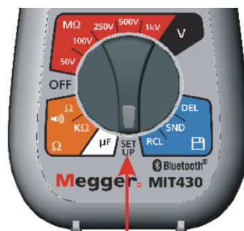
Selector switch set to Setup
