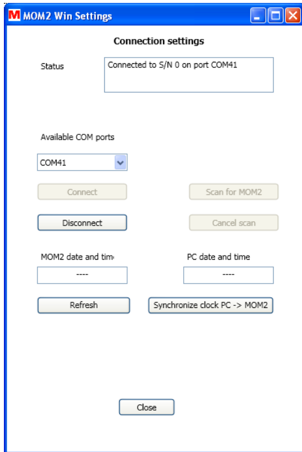
Figure 8.4.3 The Connection settings window, connection established.
