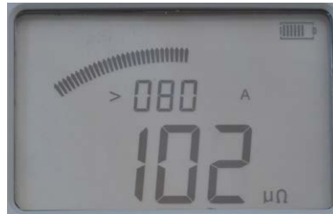
The minimum current was 80 A and the resistance value is 102 μΩ.
