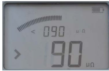
The small digits show the set P/F value (< 90 μΩ). The character ">" to the left of the big digits indicates that the P/F value was exceeded.
