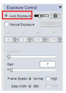
Normally Auto Exposure function can get proper brightness preview. If preview is still dark, manually set <u>Gain</u> to the middle of the slider.
