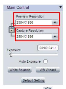
Click the Lock tag to lock/unlock the preview and capture resolution. Unlocking it allows to set different preview and capture resolution (Usually use for low resolution preview, high resolution for capture).
