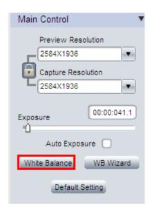
To get better white balance result, please move the sample to the blank area and then hit <u>White Balance</u> button, then move back the sample. Or also can click <u>WB Wizard</u> and follow the steps to finish the white balance.
