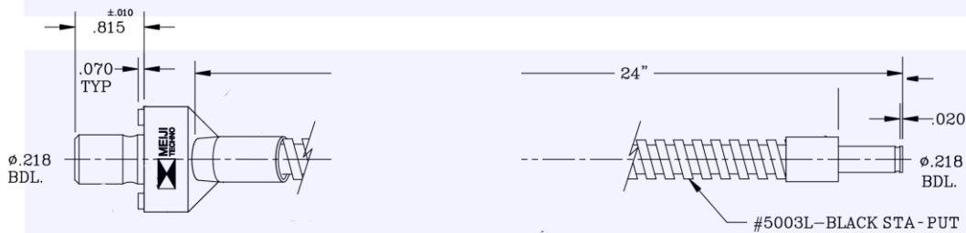
FT190/75 Single arm repositionable gooseneck light guide with black matte sta-put and SS branch tips. Accepts optional Lens (FT190/50) and Polarizing cap (FT19085).
