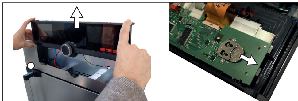
Fig. 41 Removing the lithium battery
