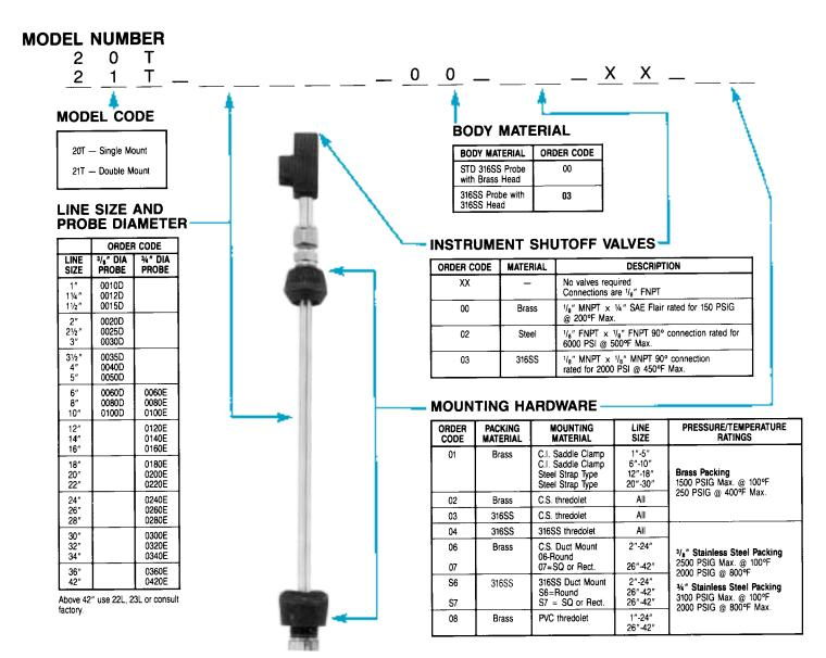
SERIES 20T—ACCUTUBE—SINGLE MOUNT. The Accutube Series 20T Standard Probe is constructed of stainless steel and brass. The Series 20T Probe has single-mounted support and installs through a single packing gland and thredolet. The Series 20T Accutube is factory-fitted with 1/8" FNPT connections and is shipped with mounting hardware complete. Series 20T Accutubes available for line sizes 1" through 30".
