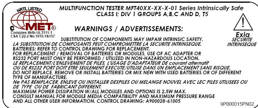
WARNING label for Intrinsically Safe MFT Units
