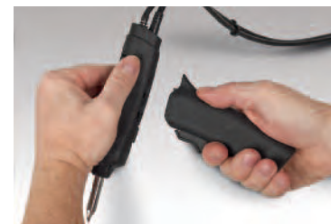
Remove grip for Pencil config.
