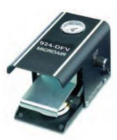
The 924-DFV Series Foot Valve Dispenser offers increased production combined with dispenser economy. Floor mounted, they have a built in pressure regulator, pressure gauge and a unique fast-dump, three-way air valve. Output rate and shot size are operator controlled.
