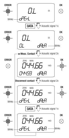
As long as the DATA function is active and all measurements are within the measuring range which has been automatically adjusted, the measuring ranges should not be changed manually.
