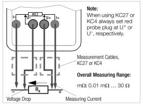
KC4 Kelvin clips and KC27 Kelvin probes (available as accessories) allow for easy, correct connection. Resistance at the current jacks should amount to  $< 1 \Omega$ .
