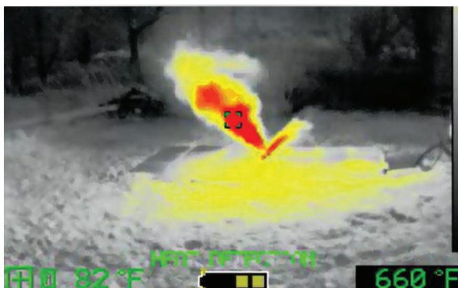
Invisible gas detected by the Mi-TIC
